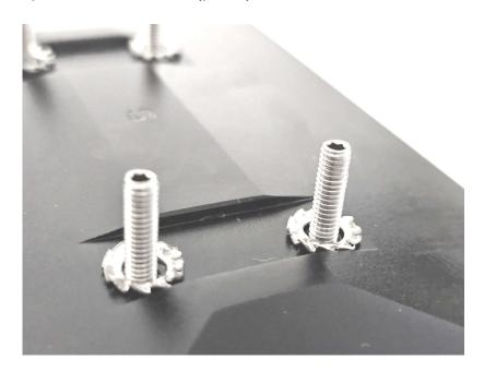
Put the shoulders in place, add another four compression washers and four hex nuts, and hand-tighten them (pic 4).
