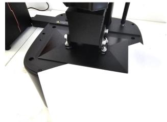
All hardware is made of AISI 304 and will not rust or react with BC resins.
