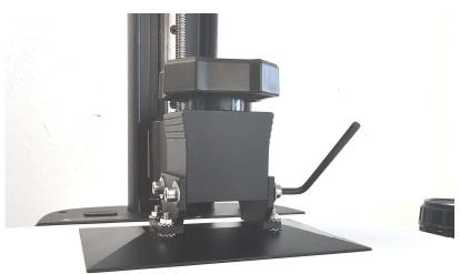
Move the paper under the platform to locate where the platform is pressing too much, and tighten the hex nut in the corresponding corner, no more than 45° each time. Check again with the paper (pic 8).
