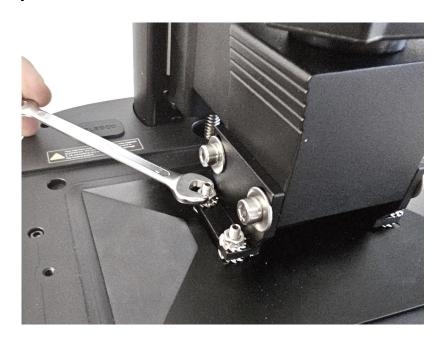
Repeat the Z zero process, but this time, do not loosen the screws and remove the paper to return the Z-axis to its proper home position.
